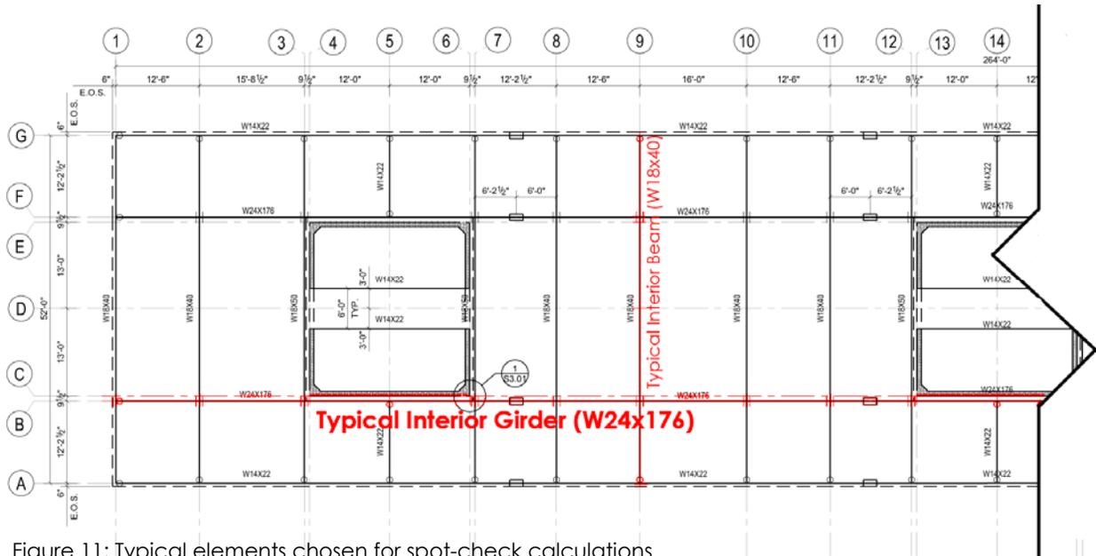
Figure 11: Typical elements chosen for spot-check calculations
