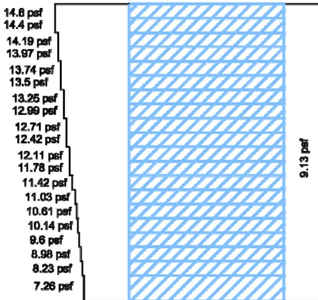
Figure 8: North-South Direction Wind Pressures
