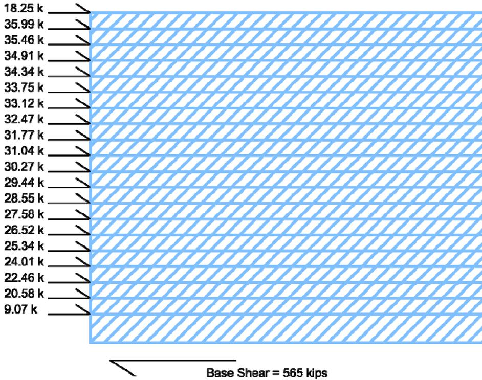
Figure 9: East-West direction wind forces at each story
