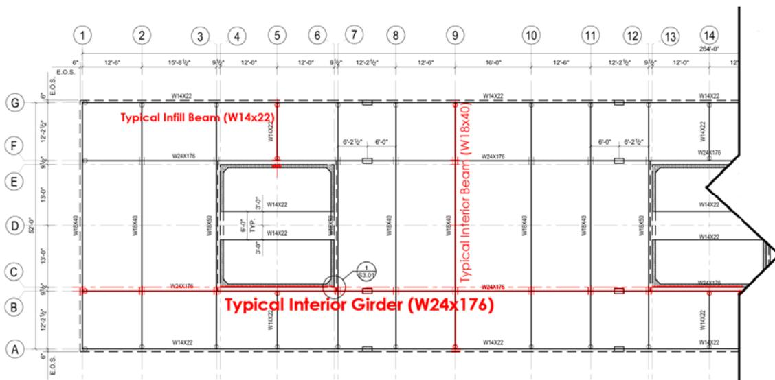
Figure 3. Typical framing plan (building's symmetric about line 7).
