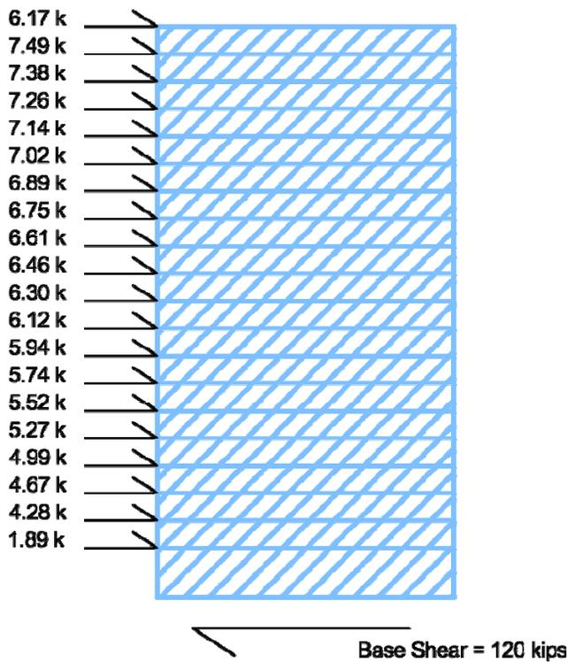
Figure 10: North-South direction wind forces at each story
