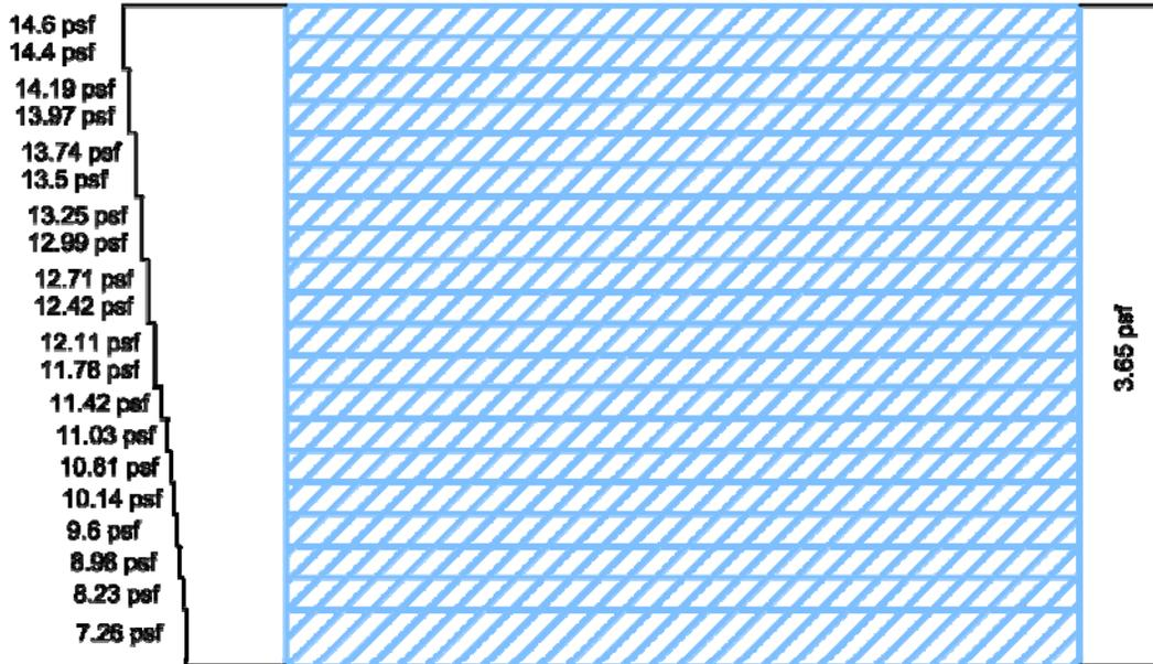
Figure 7: East-West Direction Wind Pressures
